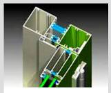
Will accept hinged, pivot or sliding doors. Doors are 50mm thick. Heavy duty adjustable hinges with extruded aluminium backing plates designed to support heavy door panels. The wide stiles allow us to fit wide backset locks.
