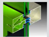
Designed to accept 24mm IGUs. Glazing pocket offers I2mm glass bite on Insulating Glass Units (IGUs). A variety of pocket closer extrusions are available should monolithic glass be required.
