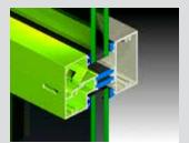
Designed to accept 24mm IGUs. Glazing pocket offers the required 12mm glass bite on IGUs. A variety of pocket closer extrusions are available should thinner glass be required.
