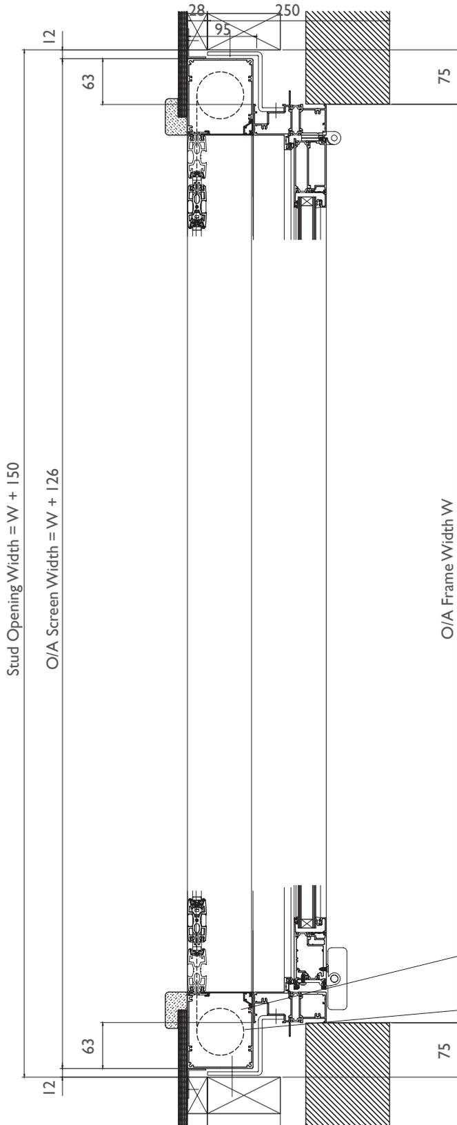
Bi-fold doors with unequal number of panels using a single screen have to be less than 4485mm wide with Standard weave mesh.
