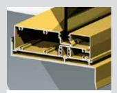
I50mm offset glazing that maintains glazing line to Series 400 and 80 suites. Sub-sill has additional support leg under glass, to carry weight of heavy glass preventing frame dishing.
