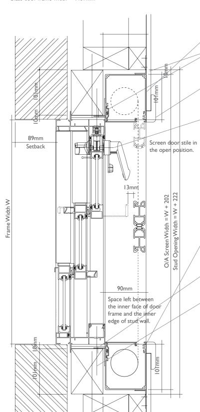
Gyprock secured to stud wall and flydoor jamb with fast grab flexible sealant.
