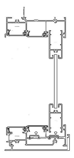
This detail shows how the sub-sill could be cut down to suit a flat sill detail.
