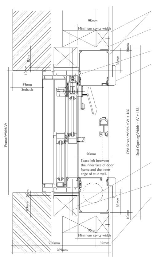
Gyprock secured to stud wall and flydoor jamb with fast grab flexible sealant.
