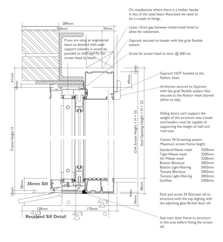
Important Note: The wall is 289mm thick excluding the internal wall lining.
