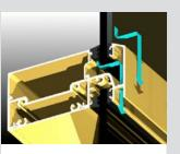
Concealed drainage designed to shed water more efficiently. Very high water performance 600 Pa.
